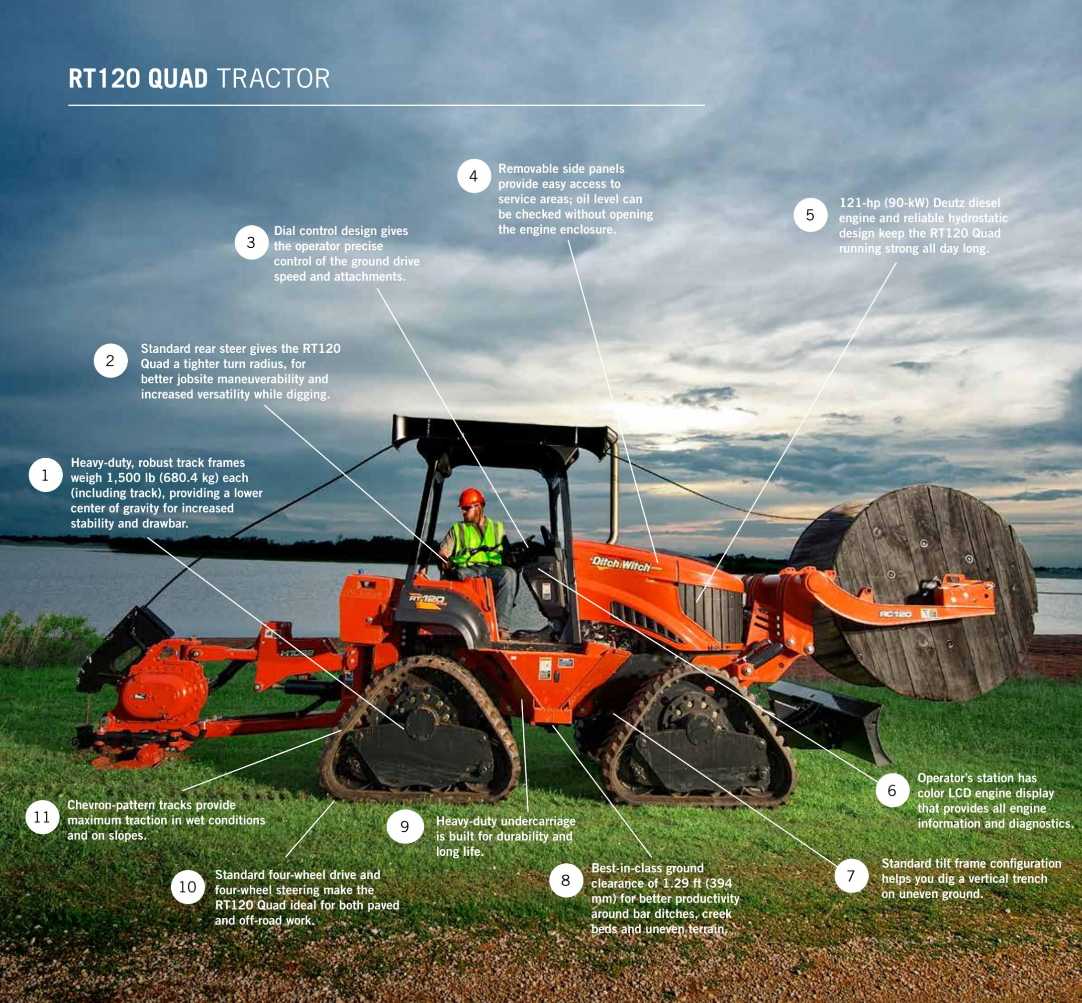
1 Heavy-duty, robust track frames weigh 1,500 lb (680.4 kg) each (including track), providing a lower center of gravity for increased stability and drawbar.
